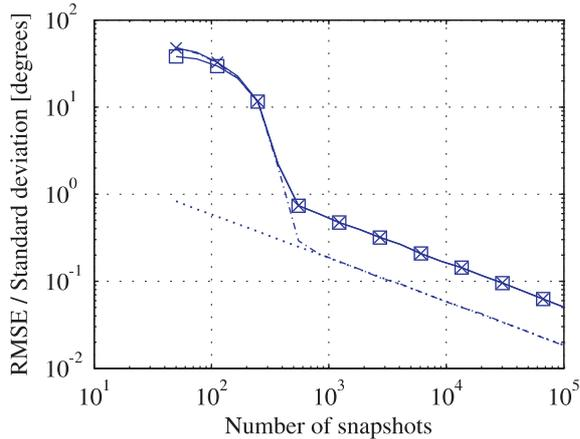
**Fig. 2.** DOA estimation performance for more sources than sensors. Solid line with crosses: RMSE of the FDCA estimates. Solid line with squares: Standard deviation of the FDCA estimates. Dash-dotted line: RMSE of the refined FDCA estimates, based on a local maximization of the likelihood function. Dotted line: Stochastic CRLB.
