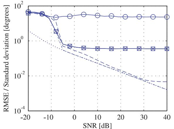
**Fig. 3.** DOA estimation performance in the case of manifold ambiguities. Solid line with crosses: RMSE of the FDCA estimates. Solid line with squares: Standard deviation of the FDCA estimates. Dash-dotted line: RMSE of the refined FDCA estimates, based on a local maximization of the likelihood function. Dashed line: RMSE of the Capon estimates. Solid line with circles: RMSE of the MUSIC estimates. Dotted line: Stochastic CRLB.
