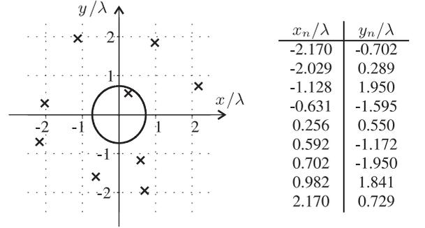
**Fig. 1.** Array geometry (the sensor locations are depicted by the crosses). The circle shows as a reference the size of a UCA with the same number of sensors and  $\lambda/2$  spacing between adjacent sensors.
